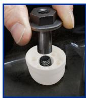
Easier to install than traditional sway bar link kits, the MOOG Problem Solver bolt style sway bar link features patented molded bushings that center and hold the coated washers in place, making them easier to install. Instead of a standard nut, MOOG sway bar link kits use a 1"-barrel lock nut that can easily be threaded on, even if the bolt end is flush with the washer. This saves time during installation.
