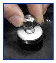
MOOG PROBLEM SOLVER BARREL LOCK NUT MAKES INSTALLATION EASIER
