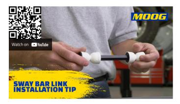
When installing MOOG bolt style sway bar links (also called barrel lock nut), it is important to avoid overtightening the bolt. MOOG bolt style sway bar links feature a self-locking barrel nut on the end of a polyurethane bushing that doesn't compress like a standard bushing when it is tightened.
